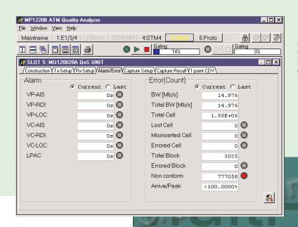
Non-conforming ATM Cell which exceed the bandwidth allocation of the GCR Algorithm can be detected by the MP1220B.
