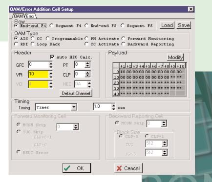
The OAM test cell utilized by the MP1220B QoS unit can be defined for F4 and F5 test flows where both error injection and detection can be realized.
